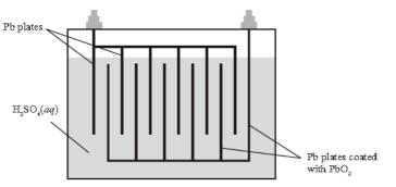
The reactions occurring when the battery is operating are:
